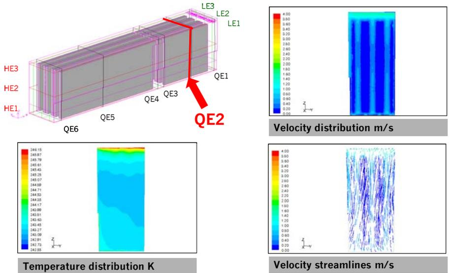
In this transverse section, note the distinct air speed down the length of the room as air flows from the air coolers to the opposite side of the room. (Figure 10) Some of the warmed air flows upward, forms a thin layer under the ceiling and flows back to the coolers.
