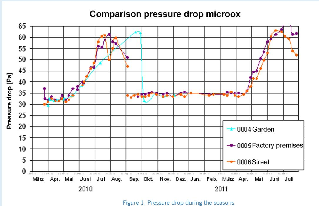
During the experiment, no noticeable difference was registered in the soiling characteristics of the two heat exchanger technologies. Indeed, the microox® heat exchangers reached the maximum admissible pressure drop about two weeks before the finoox® heat exchang-
